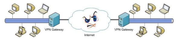
Figure 2. Gateway-to-Gateway Architecture
